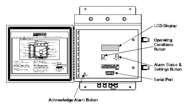
Figure 3-10: Serial Port Location
